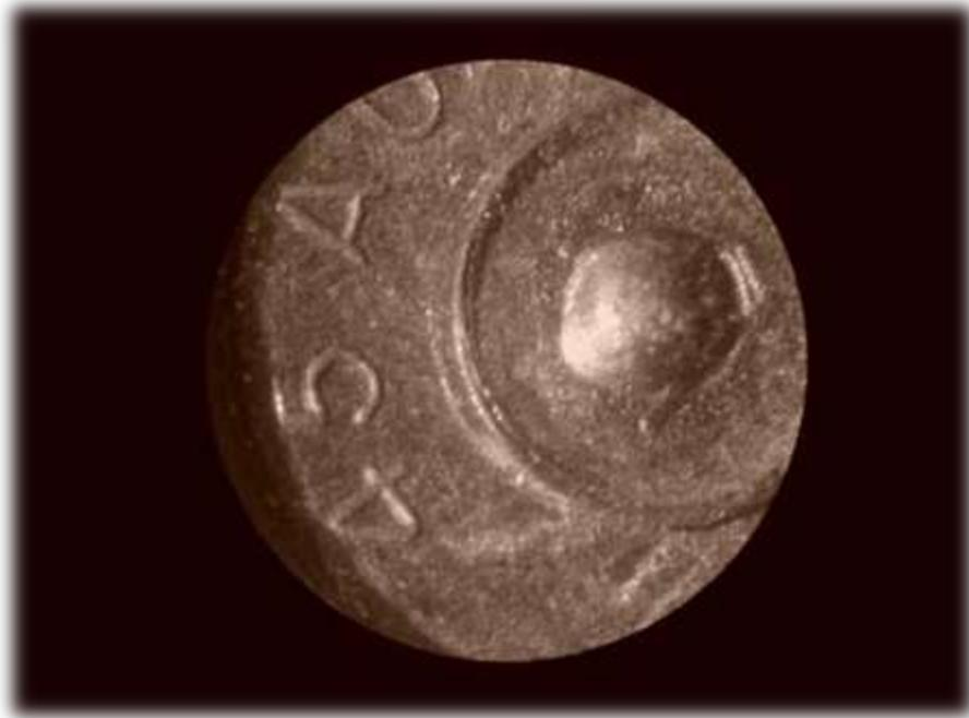
*Viewing the hologram of the spent bullet shell through one of the eyepieces of the 3D stereo microscope. Through the microscope one can see the depth that would be present if the actual bullet shell were there instead of the hologram.*
